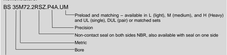
BS = single ball screw bearing, BSD = double row without flange, BSDF = double row with flange We also have our IBC Ball Screw support Bearings available in inch sizes.
